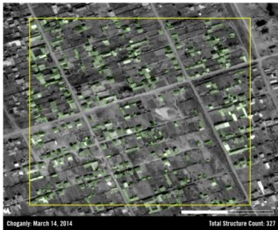
FIGURE 2: A 0.25 square kilometre area within Choganly neighbourhood. In the March 2014 image, 327 structures can be seen, outlined in green below. In the April 2015 image, 207 structures appear to have been demolished (outlined in red) and only 120 of the previous structures remain.
